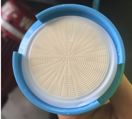
Figure 2: Week 1 SDI membrane result from R.O feed
