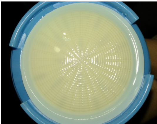
Figure 1: Week 1 SDI membrane result UF system
