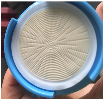
Figure 3: Week 2 SDI membrane for the R.O feed system
